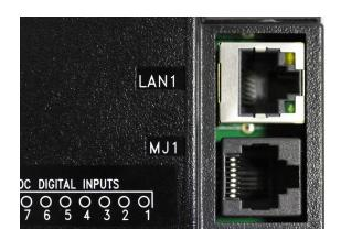
Figure 10.2 – MJ1 Connector to be used via Serial or with Serial to USB adapter to PC
